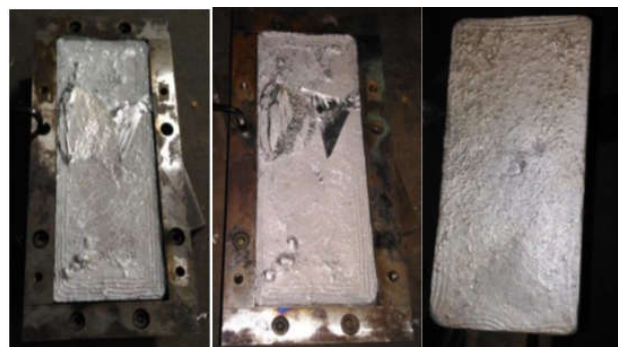
Fig 2. Cast specimens (15%,20% and 25% Fly Ash)
