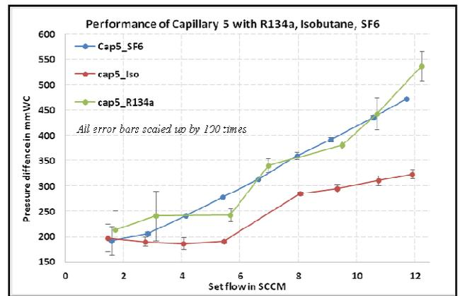
Figure 7. Capillary C5 Results with R134a, Isobutane and SF6 gases
