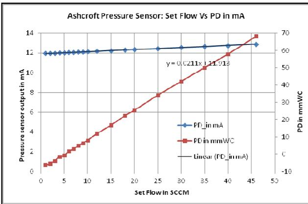
Figure 5. Ashcroft Pressure Sensor: Out 4mA to 20mA
