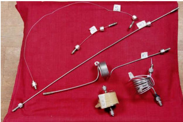
**Figure 1. Various Capillaries: C2, C5 and C6: 300 micron (ID); C1, C3, and C4: 1800 micron (ID)**
