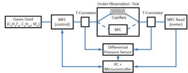
**Figure 2. The Experimental Setup**
