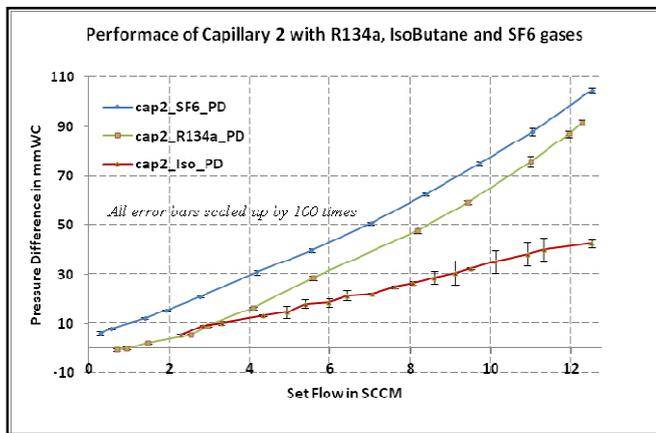
Figure 6. Capillary C2 Results with R134a, Isobutane and SF6 gases
