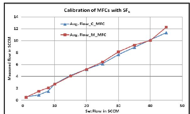
**Figure 3. SF6 MFC Calibration**
