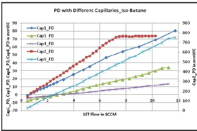
Figure 4. Result with Ashcroft Differential Pressure Sensor
