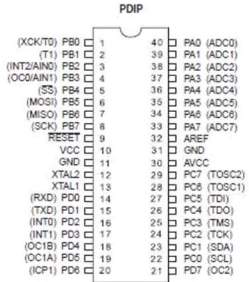
Figure 4.2.1. Showing Pin Out of ATMEGA 16
