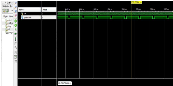
Fig. 11. Timing diagram of PWM
