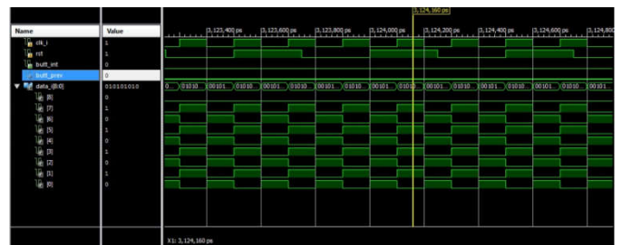
Fig. 17. Timing diagram of Interrupt controller
