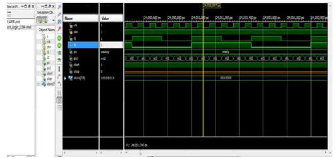
Fig. 8. Timing diagram of UART
