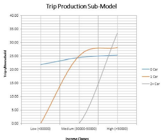
Figure 4. Trip Production Sub-model
