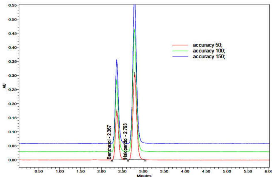
**Figure 5. Accuracy overlay chromatograms of Haloperidol and Benzhexol**
