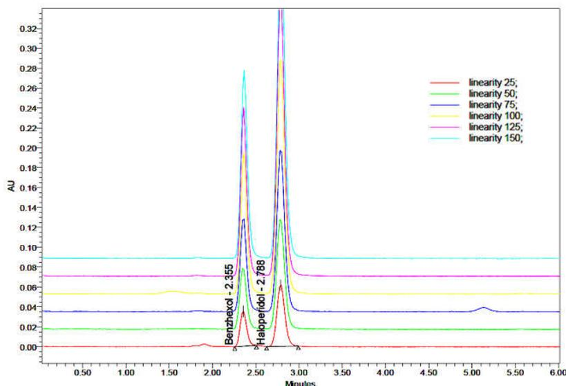
**Figure 4. Linearity overlay chromatograms of Haloperidol and Benzhexol**
