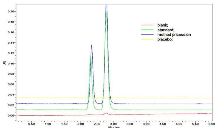
**Figure 3 (c). Specificity overlay chromatogram of blank, standard, placebo and marketed sample of Haloperidol and Benzhexol**
