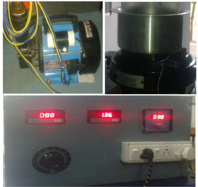
Figure: voltmeter, ammeter, temperature indicator, dimmer stat, glass cylinder, pump, heater with aluminium bowl, control panel.
