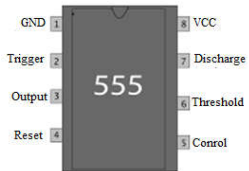
Fig.13. Pin Diagram of IC ne555
