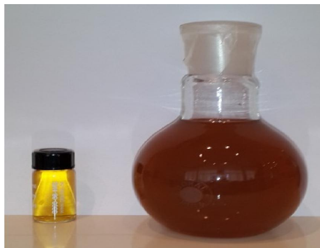
Fig.2. Extract from the Pomegranate leaves: on the right– 1.0 ml \text{AgNO}_3 solution of 10^{-2}\text{M} concentration is added to the extract
