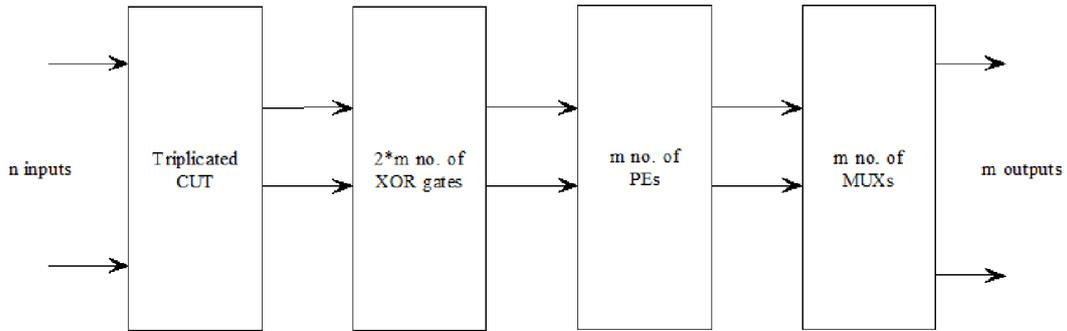
Fig. 1 lock diagram of the self healing decoder
