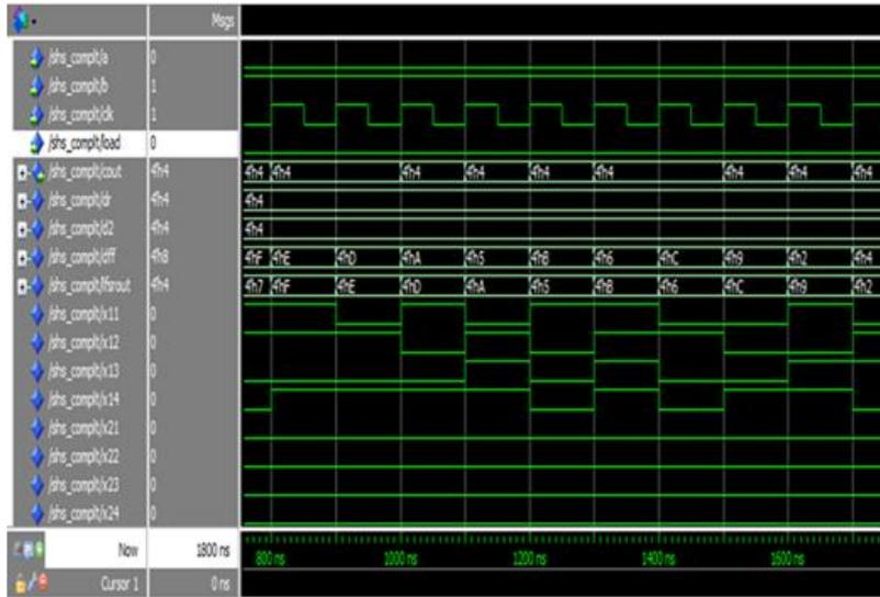
Fig. 4. Output of the self healing system with faults in the output lines of the first decoder
