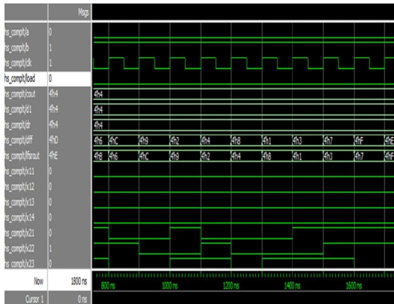
Fig. 5. Output of the self healing system with faults in the output lines of the second decoder
