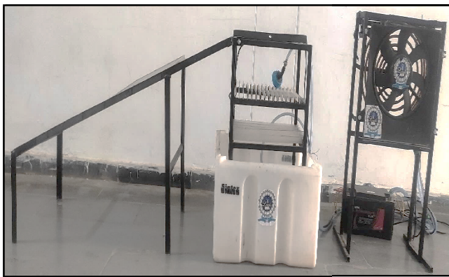
Fig. 5. Solar Evaporative cooling system
