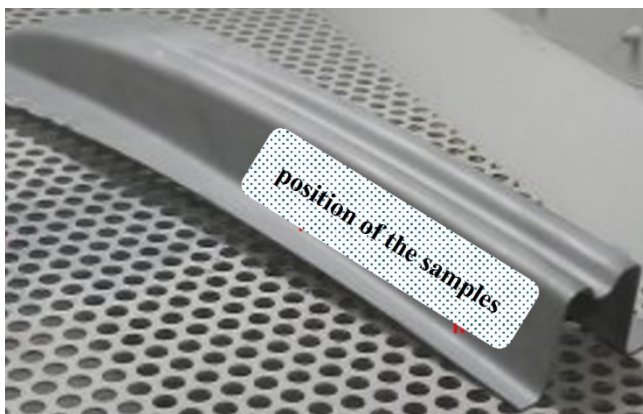
Figure 3. Position of samples for simulation and tensile tests
