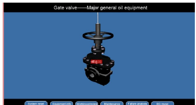
Fig. 2. Major general oil equipment, the gate valve
