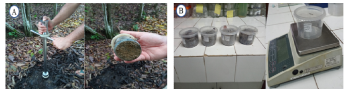
Figure 2. Metal probe used to collect soil samples at a depth of 0-10 cm (A). Weighing of soil samples to obtain the water content retained in the sample (B) (2019)
