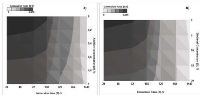
Figure 3. Variation of CR with a) additive concentration and the immersion time, fixing biodiesel concentration at 20%; b) biodiesel concentration and the immersion time, fixing additive concentration at 1%
