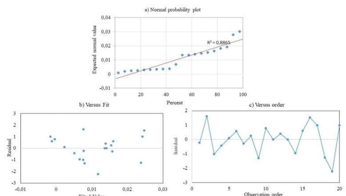
**Figure 1. Residual plots for CRs of steel showing the accuracy of the model used**
