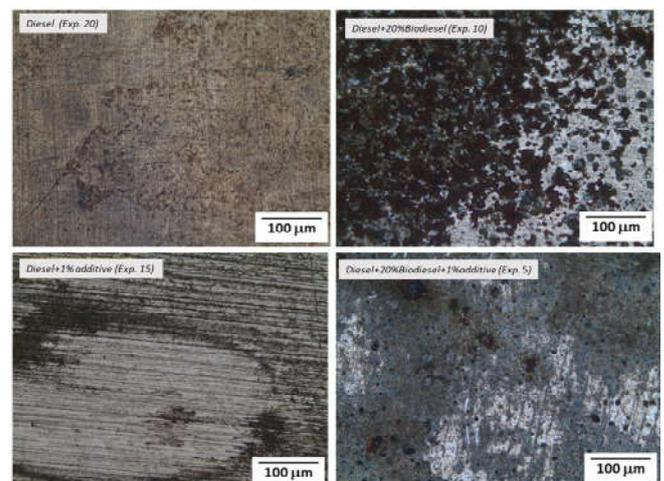
Figure 4. Optical images of microalloyed steel specimens after 1440 h immersed in fuels mixture
