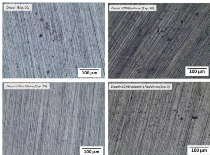
**Figure 5. Optical images of microalloyed steel specimens after 1440 h immersed in fuels mixture and subsequent sanding**
