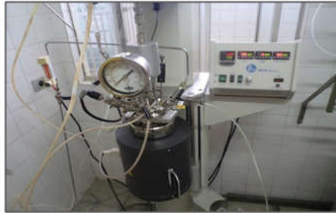
Figure 2. Slurry reactor PARR 4848 used for catalytic oxidations performed in this work
