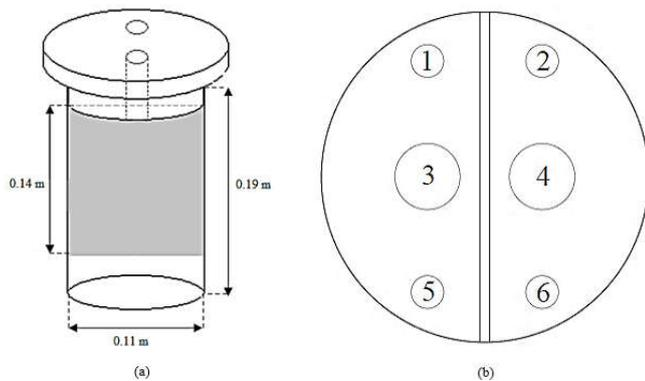
**Figure 1. The electrolytic cell built: (a) Front view and (b) Upper view with: (1) H<sub>2</sub> gas output, (2) O<sub>2</sub> gas output, (3) cathode; (4) anode; (5) water inlet and (6) thermometer input**
