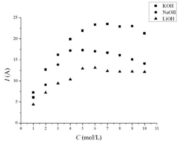
**Figure 4. Electric current ( $I$ ) as function of the concentration ( $C$ ) of KOH (■), NaOH (●) and LiOH (▲)**
