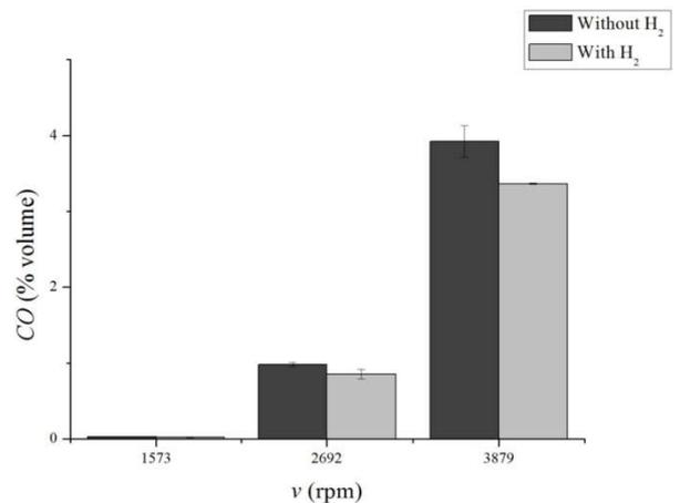
**Figure 7.** Variation of the emissions of carbon monoxide (CO) in function of engine speed (v)
