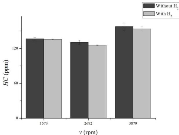
**Figure 6.** Variation of the emissions of unburned hydrocarbons (HC) in function of engine speed (v)
