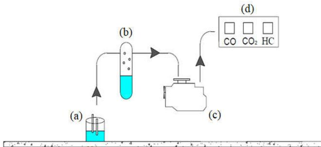
**Figure 3. General configuration of the experiments performed on the internal combustion engine with: (a) electrolytic cell; (b) bubbler; (c) engine; (d) gas analyzer**
