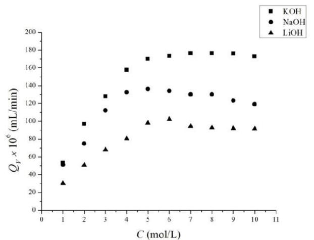
**Figure 5. Hydrogen gas flow rate ( $Q_V$ ) as a function of the concentration ( $C$ ) of KOH (■), NaOH (●) and LiOH (▲).**
