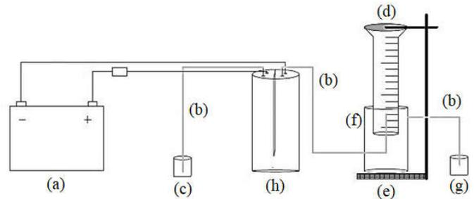
**Figure 2. Experimental unit for the flow measurement of hydrogen with: (a) automotive battery; (b) silicon ducts to output of the gases; (c) beaker containing water for O<sub>2</sub> gas bubbling; (d) graduated cylinder; (e) retort stand; (f) beaker containing water; (g) beaker to receive the water supernatant from the graduated cylinder and (h) electrolytic cell**
