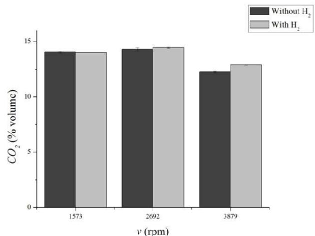
**Figure 8.** Variation of the emissions of carbon dioxide (CO<sub>2</sub>) in function of engine speed (v)
