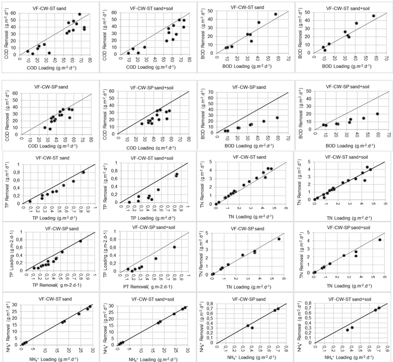
Figure 4. Applied organic loading and removed organic loading values for the parameters COD, BOD, TP, TN, and NH<sub>4</sub><sup>+</sup>
