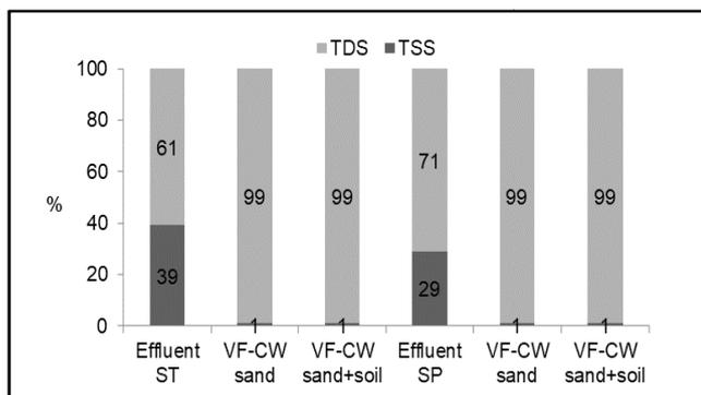
**Figure 3. Total, suspended, and dissolved solids percentage distribution in the raw effluent and post the constructed wetlands treatment**
