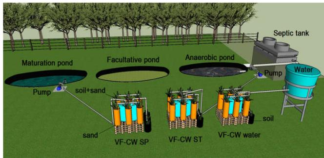
Stabilization pond (SP): Anaerobic Pond (AP) + Facultative Pond (FP) + Maturation Pond (MP); VF-CW SP: vertical flow constructed wetland for stabilization pond effluent treatment; VF-CW ST: vertical flow constructed wetland for septic tank effluent treatment
