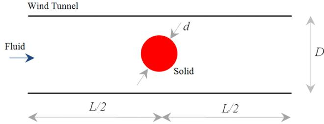
**Figure 1. Schematic view of the wind tunnel with  $d$ ,  $D$  and  $L$  equal to 0.02, 0.20 and 0.40 m, respectively**
