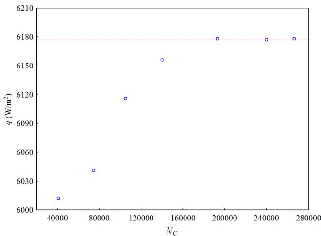
**Figure 3. Grid independence test to determine the number of computational cells**
