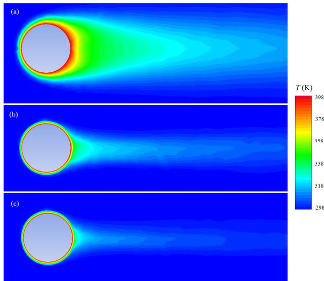
**Figure 7. Air thermal distribution ( $Pr = 0.71$ ) around the sphere for different flow regimes: (a)  $Re = 100$ , (b)  $Re = 5050$  and (c)  $Re = 10000$**
