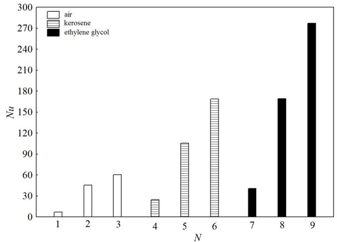
**Figure 8. Nusselt numbers obtained via CFD from the combination of *Prandtl* and *Reynolds Numbers* of the Design Matrix (Table 1)**
