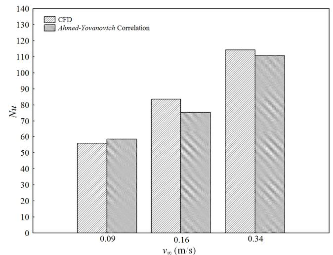
**Figure 5. Mean values of Nusselt Number estimated by CFD techniques and by the Ahmed-Yovanovich Correlation for water at 298 K**
