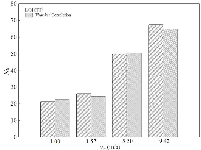
**Figure 4. Mean values of Nusselt Number estimated by CFD techniques and by the Whitaker Correlation for air at 298 K**
