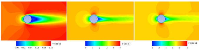
**Figure 6. Air velocity profiles ( $Pr = 0.74$ ) around the sphere for different flow regimes: (a)  $Re = 100$ , (b)  $Re = 5050$  and (c)  $Re = 10000$**
