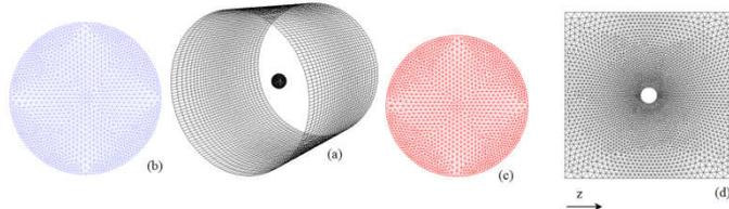
**Figure 2. Wind tunnel geometry illustrating the details of the mesh structure: (a) wind tunnel walls, (b) entry section, (c) output section and (d) cross section**
