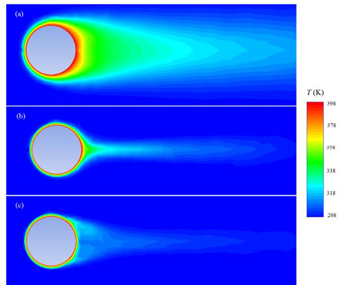
**Figure 9. Thermal distribution around the sphere for different fluids at  $Re = 100$ : (a) air, (b) kerosene and (c) ethylene glycol**
