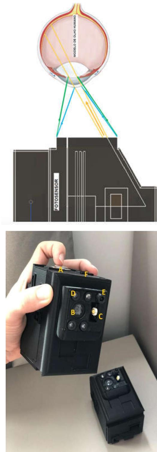
Figure 1. Operating diagram of the portable device (left) and photograph showing the grip (right)
