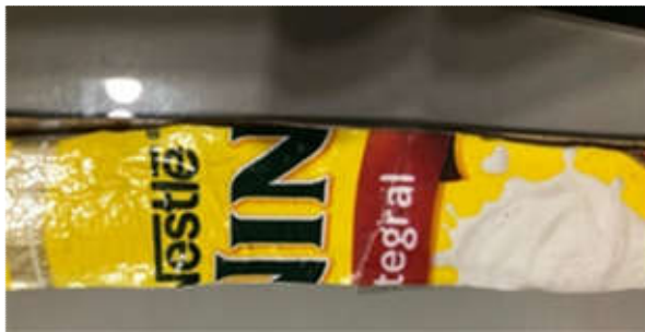
Figure 5. Samples kept outdoors without using finishing black paint in decomposing and wrinkled (AUTHOR, 2021)
