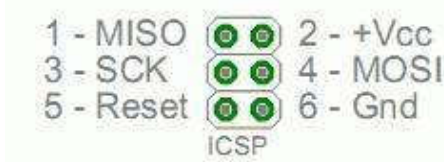
Figure 39. Arduino's SPI bus pinout
