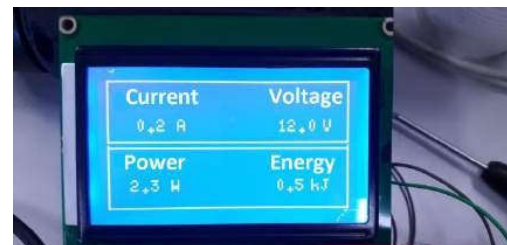
Figure 33. LoRa system interface for measurement control
