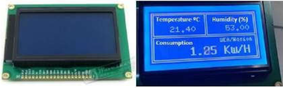
Figure 40. LCD12864 ISP interface with the Arduino Nano
