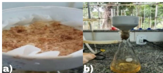
Figure 1. Filtration processing using the vacuum system to separate the extract solid from the extracting solvent after 10 days of maceration
