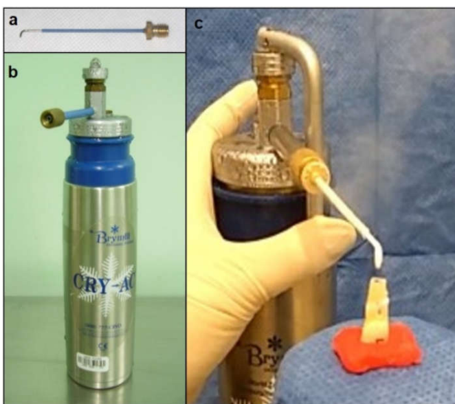
Figure 1. a) Bent spray cryoprobe Model #103-20; b) Portable cryogenic device (CRY-AC-3); c) N 2 sprayed 1 mm from the root apex
