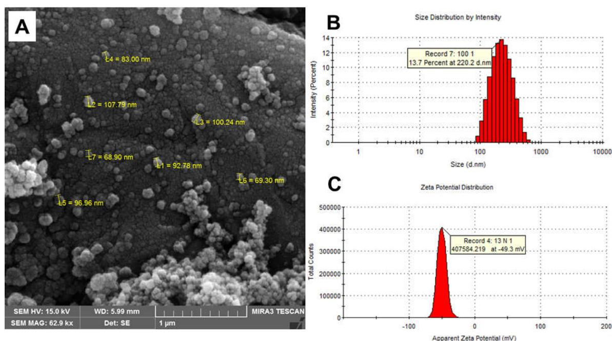
**Figure 1. Basic characterization of NLNs. (A) The NLN morphology under SEM, (B) size distribution, and (C) zeta potential determined by DLS**
