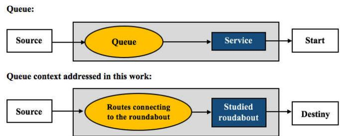
**Figure 1. Adopted queue model for representing a vehicle traffic queue**
