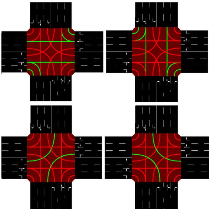
Figure 9. Traffic light stages adopted for the simulation of alternative intersection
