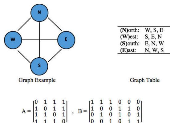
Representation of the Graph in Matrix. Matrix Adjacency (A) and Matrix Incidence (B)
