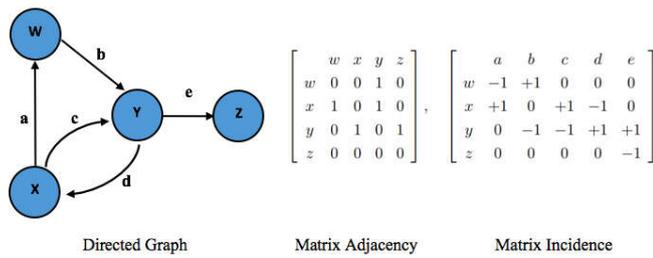
**Figure 3. Directed graph used to represent directions of traffic on roads**
