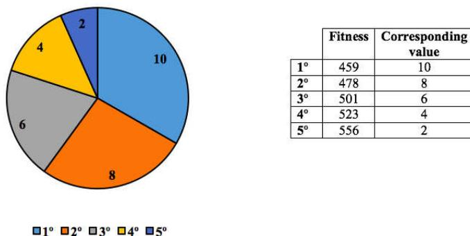
**Figure 11. Simplified example of performing the roulette technique**
