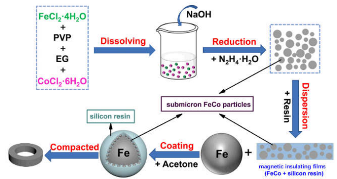
Figure 5. A schematic illustration for the preparation of Fe-based SMCs coated with magnetic insulating layers [36]
