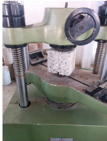
Fig.1. Compressive Strength Test
