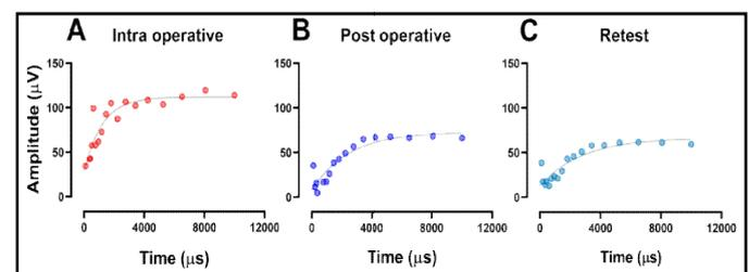
**Figure 3.** ECAP-REC functions exponential growth. (A) represents ECAP-REC  $\tau$  data, obtained during the intraoperative period. (B) shows ECAP-REC  $\tau$  data obtained after 12 months of using the cochlear implant. (C) reveals the measured stability's reliability comparing two subsequent recovery functions after 12 months using the CI device
