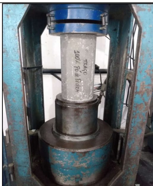
Figure 6. Trace compression test with 100% stone powder as fine aggregate
