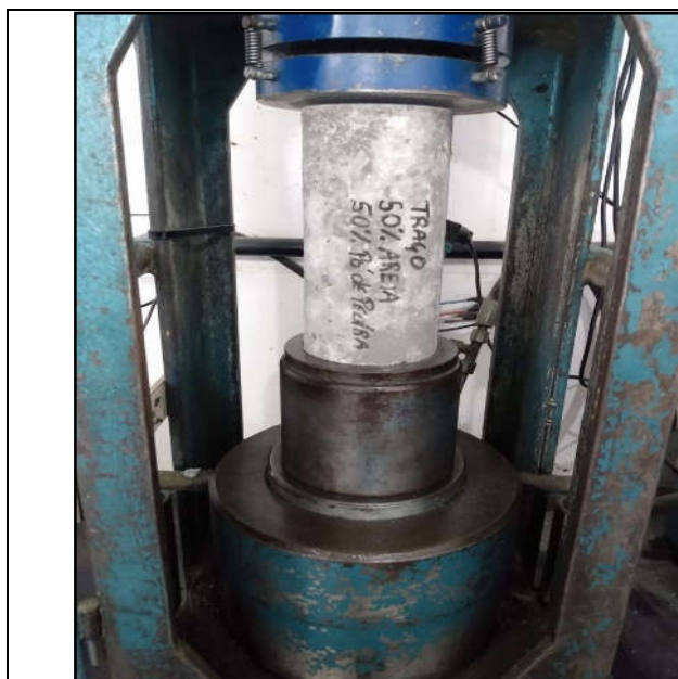
Figure 5. Trace compression test with 50% natural sand and 50% stone powder as fine aggregates
