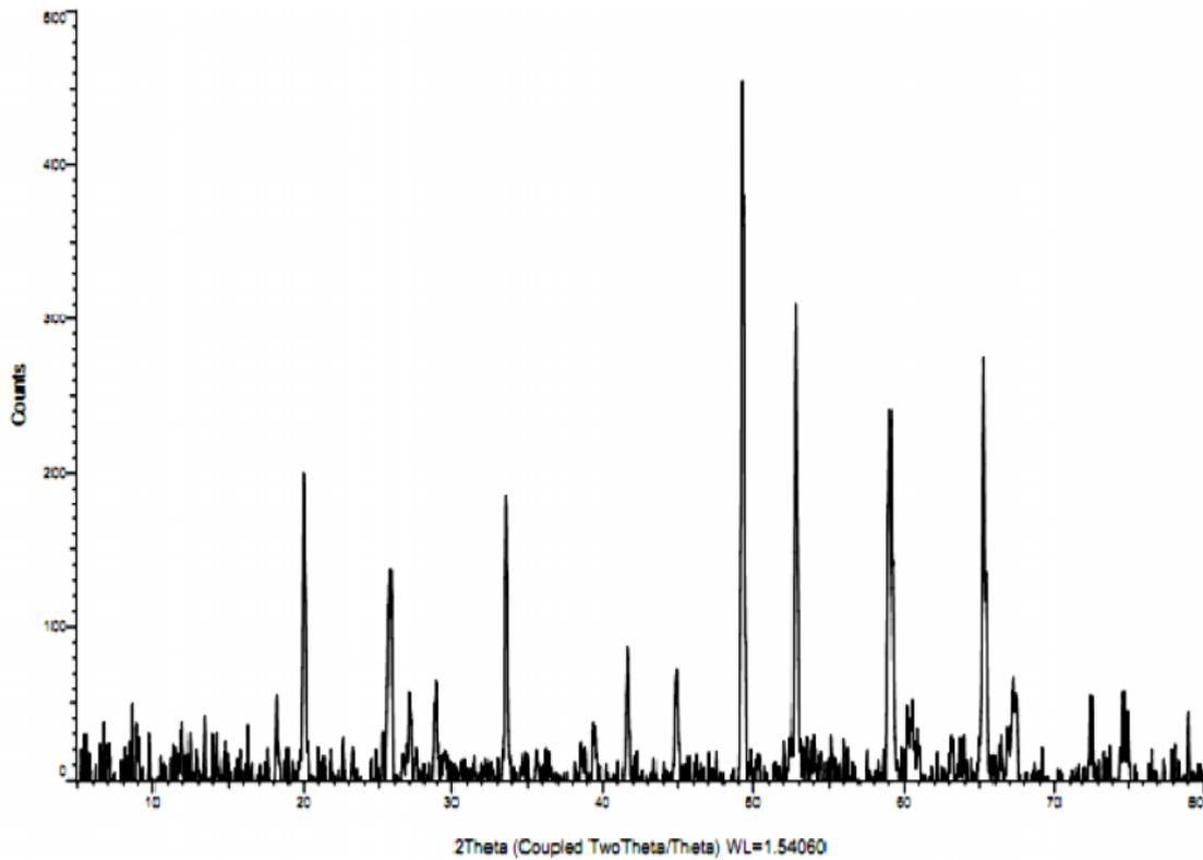
Fig. 1. XRD pattern of soil from site 1 samples (S1)
