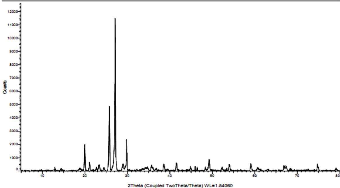
Fig. 2. XRD pattern of soil from site 2 samples (S2)
