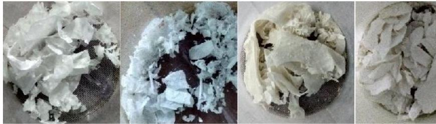
FIGURE 2. Photographic image of fibers obtained by electrospinning, (a) Without heat treatment, (b)  $\text{TiO}_2$  after heat treatment at  $650\text{ }^\circ\text{C}$ , (c)  $\text{TiO}_2/\text{WO}_3$  after heat treatment at  $650\text{ }^\circ\text{C}$  and (d)  $\text{TiO}_2/\text{Na}_2\text{WO}_4 \cdot 2\text{H}_2\text{O}$  after heat treatment at  $650\text{ }^\circ\text{C}$
