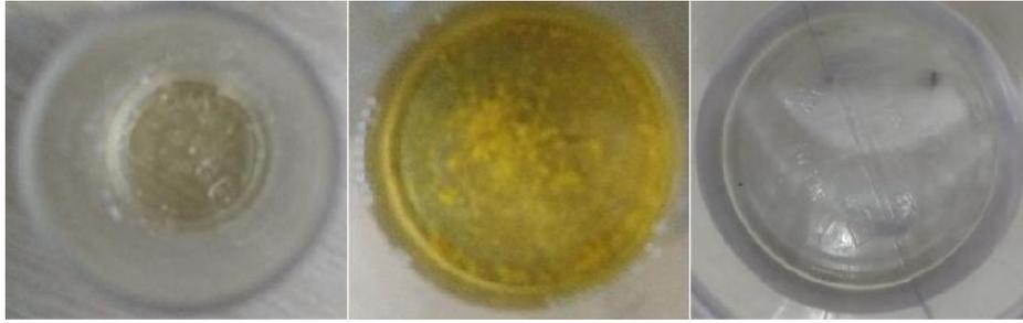
Figure 1. Color photograph of the precursor solutions for the synthesis of fibers by electrospinning, (a)  $\text{TiO}_2$ , (b)  $\text{TiO}_2/\text{WO}_3$  and (c)  $\text{TiO}_2/\text{Na}_2\text{WO}_4 \cdot 2\text{H}_2\text{O}$ , respectively
