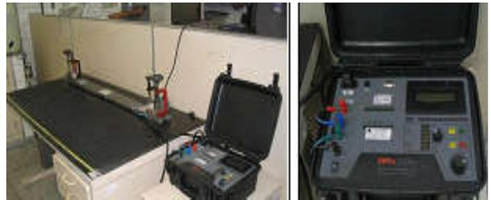
Figure 4. Photos of the Kelvin bridge components used to measure the electrical resistance
