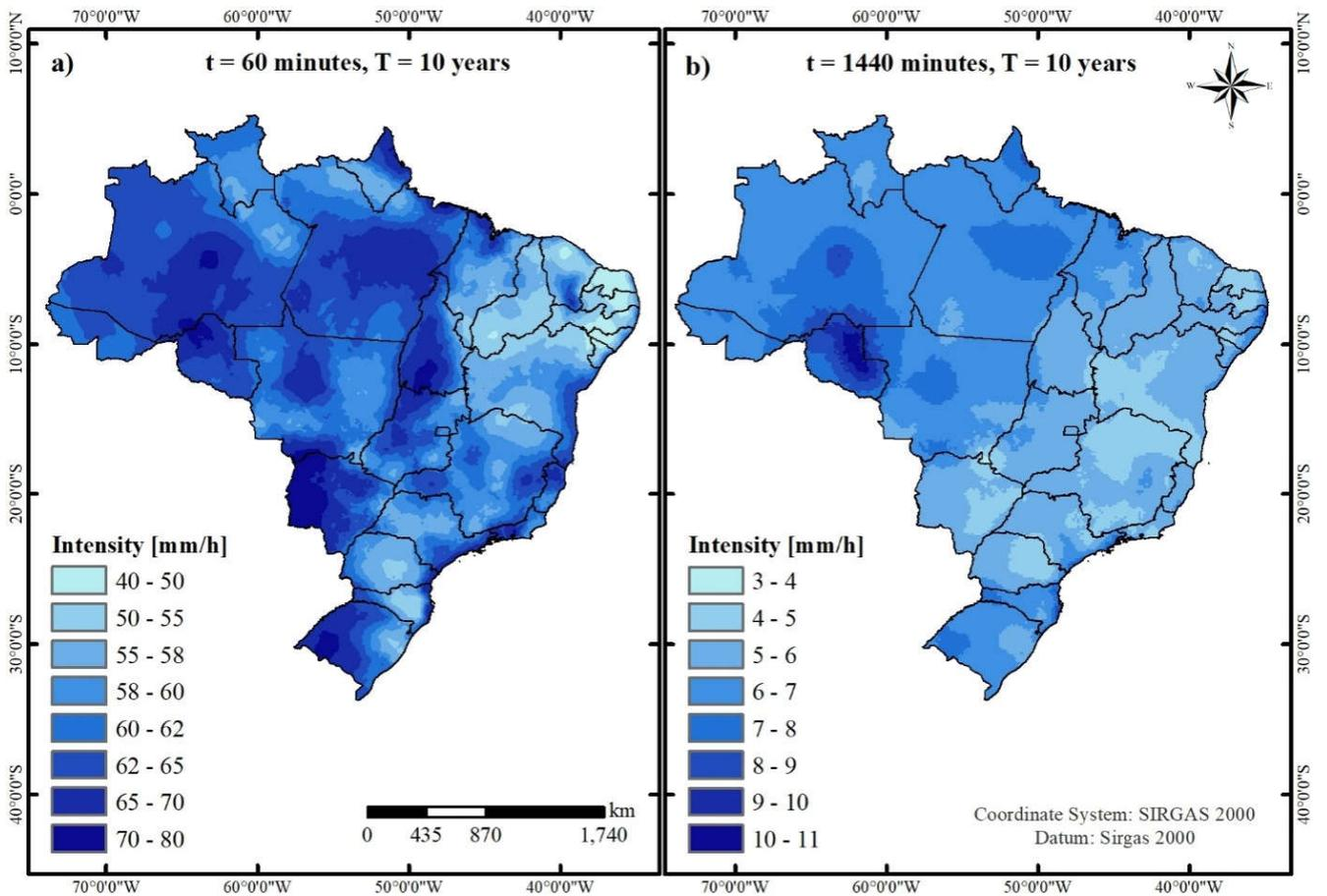
Figure 4. Maximum rainfall intensity with duration of 60 and 1440 min and a 10-year return period
