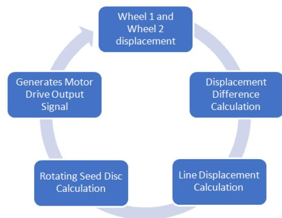
Figure 2. Firmware Line ECU
