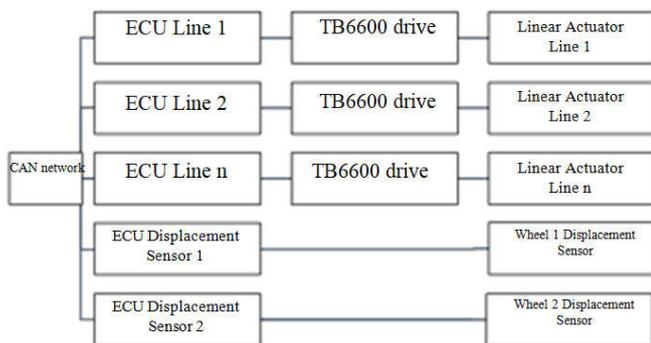
Figure 1. System Diagram
