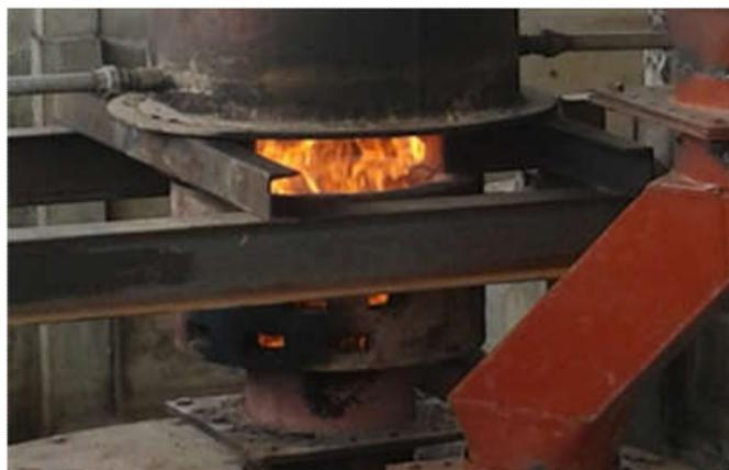
Figure 7. Feeding of a boiler by the combustion of pyrolysis gas
