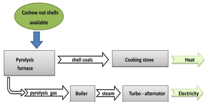
Figure 4. Synoptic diagram of the process for the sustainable energy recovery of fuels generated by the pyrolysis of available raw cashew nut shells (Kouamé Michel *et al.*, 2020)
