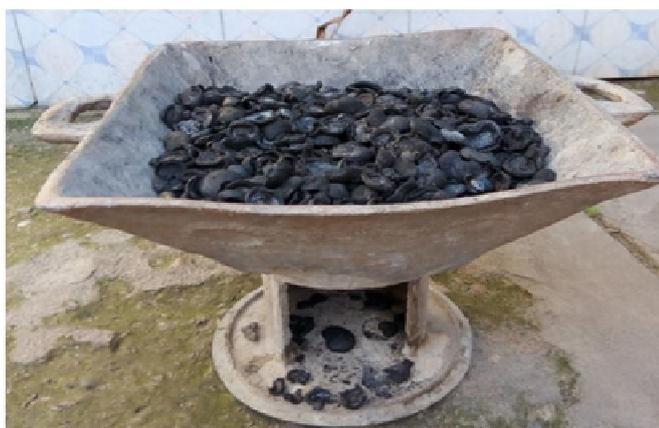
Figure 6. Upgrading of shell charcoal by means of a metallic furnace
