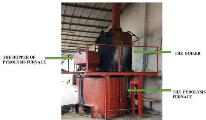
Figure 2. Example of equipment used for the thermochemical treatment of cashew nut shells (valorization of shells into pyrolysis gas for feeding a boiler)
