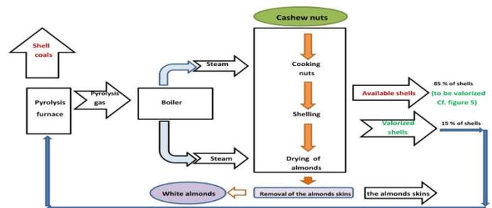
Figure 3. Synoptic diagram of the sustainable transformation process of cashew nuts using pyrolysis furnaces (Kouamé Michel *et al.*, 2020).
