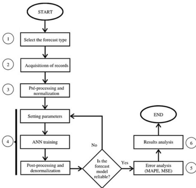
Figure 2. Load Forecasting Developed Algorithm
