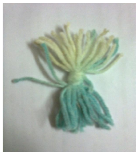
Fig. 5. Wool cloth dyed directly by dipping in a hot solution of Malachite green dye
