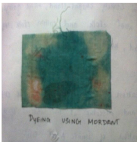
Fig. 7. The colour of cotton cloth dyed directly using mordant and then by dipping in hot solution of Malachite green
