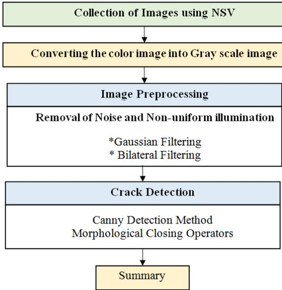
Figure 1. The study approach for detecting the fatigue cracking
