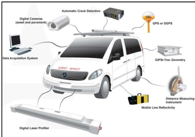
Figure 2. The Hawkeye 2000 Network Survey Vehicle
