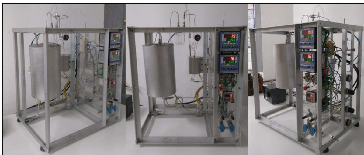
Figure 6. Assembled bench-scale test unit (450 mm wide, 550 mm long and 600 mm high)
