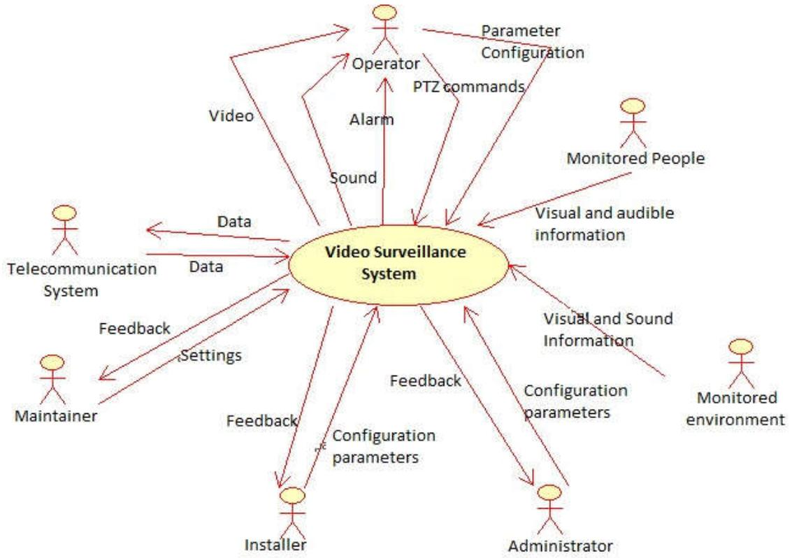
Figure 18. Product - DFD representing the video surveillance system and its relationship with the environment
