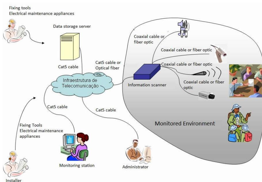
Figure 21. Product - FBD architecture interconnection diagram for a video surveillance system
