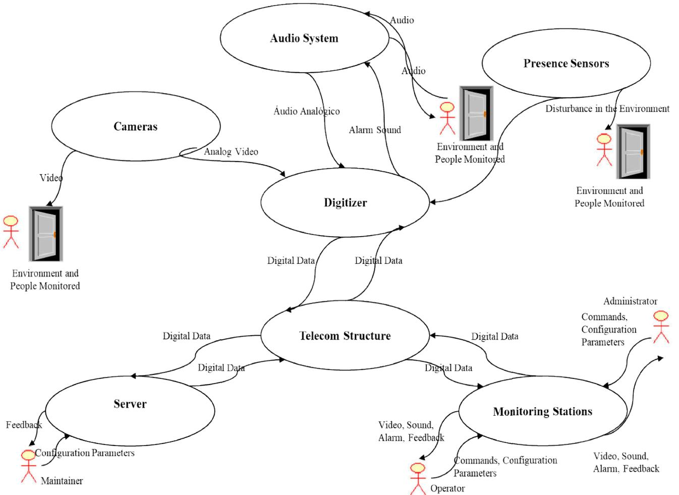
Figure 19. Product - Architecture flow diagram of the video surveillance system
