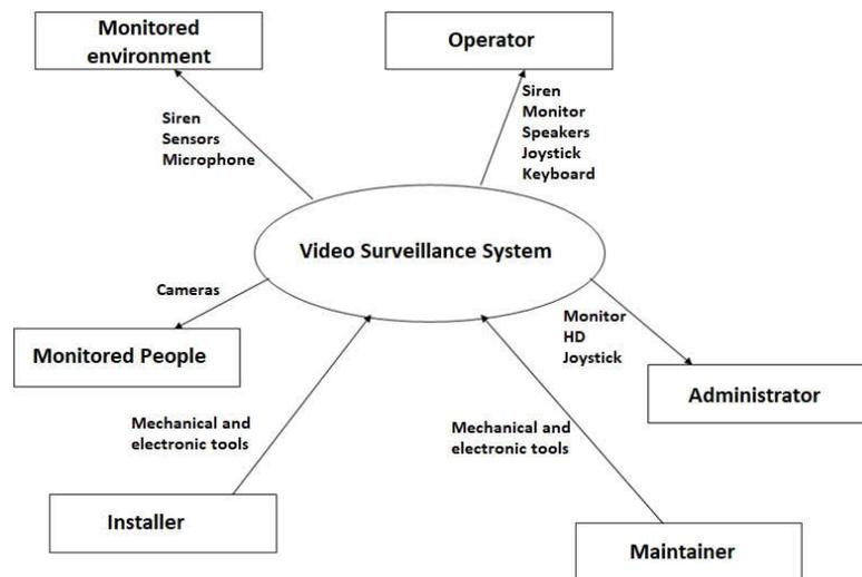
Figure 20. Product - FBD representing a monitoring system and its physical interfaces with the environment
