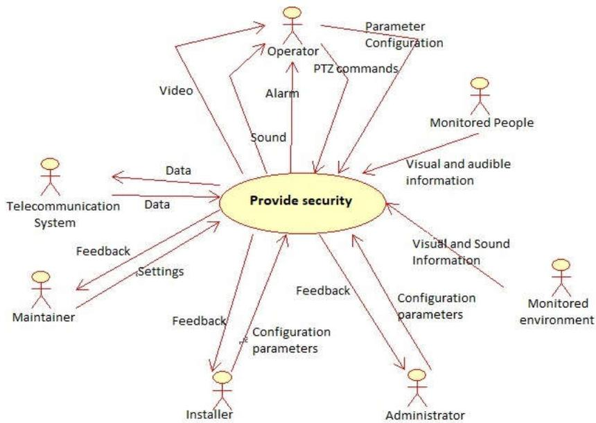
Figure 12. Video surveillance system context diagram
