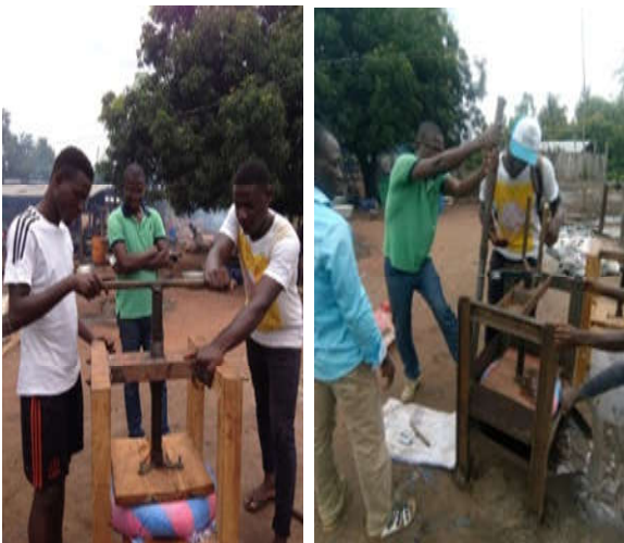
Photo 3. Pressing the cassava pulp with the two types of press
