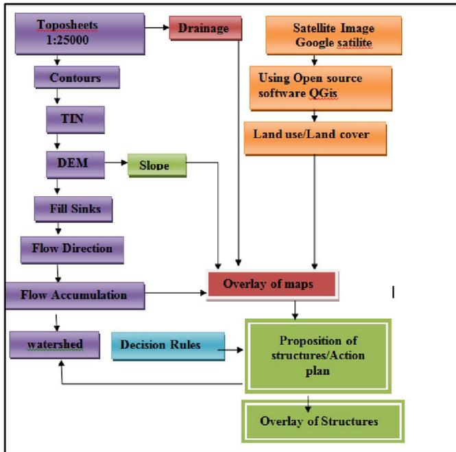
Fig. 1. Preparation plan Diagram
