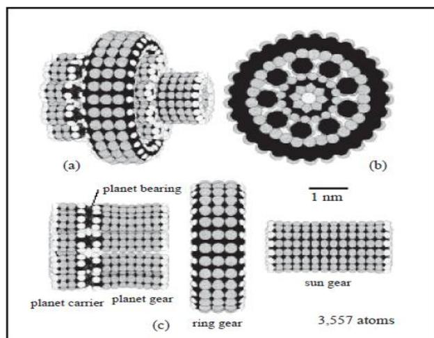
**Fig. 4: End-, side-, and exploded-view of a 3557-atom planetary gear.**<sup>15</sup> Image courtesy of K.Eric Drexler.© 1992, John Wiley and Sons, Inc.
