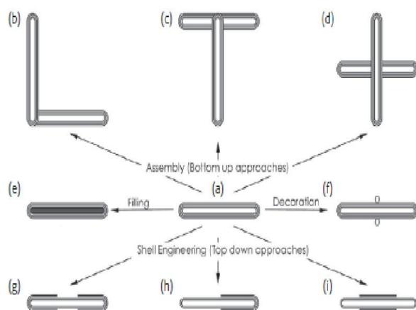
**Fig. 1.** CNT-based building blocks. Starting from (a) as-grown CNTs, nanostructures can be created by the bottom-up approaches of (b–d) assembling, (e) filling, or (f) decorating them, or in a top-down fashion by (g–i) engineering their shells/caps.<sup>7</sup>
