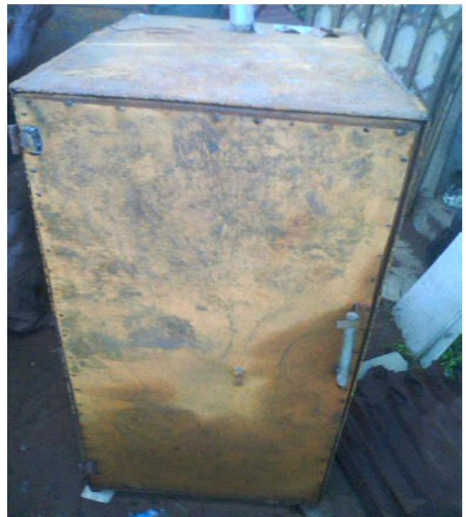
Fig 3: The Fabricated Grain Dryer
