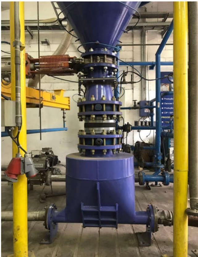
Figure 2. Batchpump prototype
