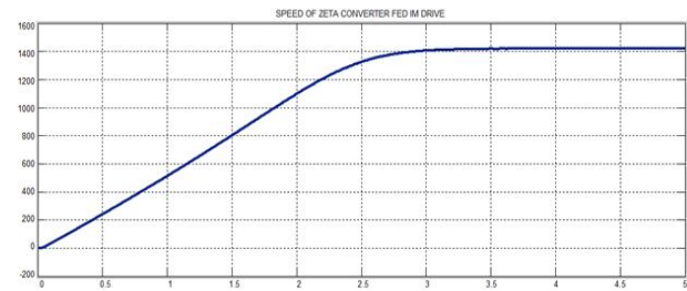
Fig. 13. Speed response of Zeta converter fed IM drive
