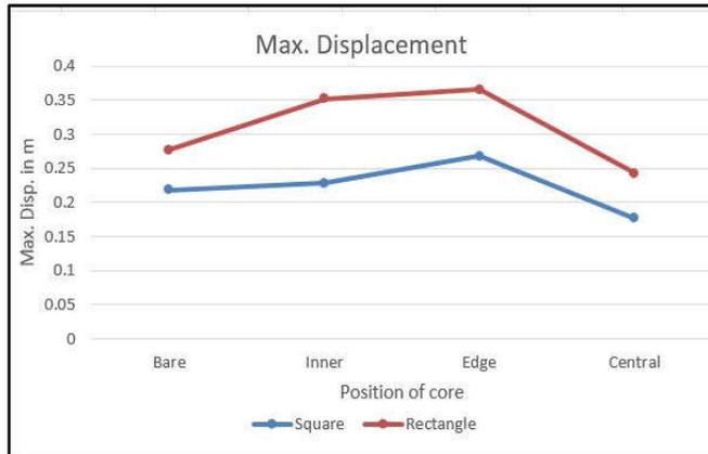
Fig. 2. Graph of Max. Storey Displacement
