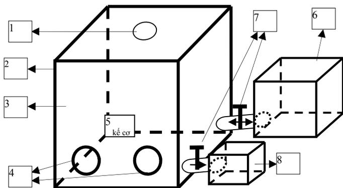
1. Top surface for placing equipments (temperature-humidity and oxygen sensors)
