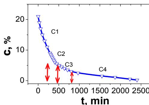
**Fig. 4. Oxygen concentration (C, %) variation as a function of oxygen reduction time (t, min), the ratio: 3g FOCOAR / L**
