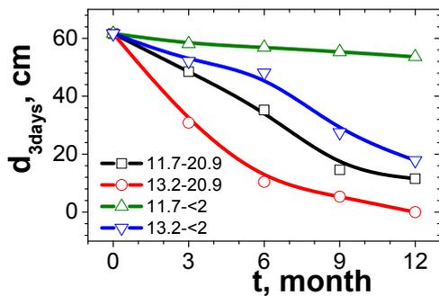
Fig. 6. Variation of  $d_{3days}$  as a function of preservation time, the same notation for Figure 5.
