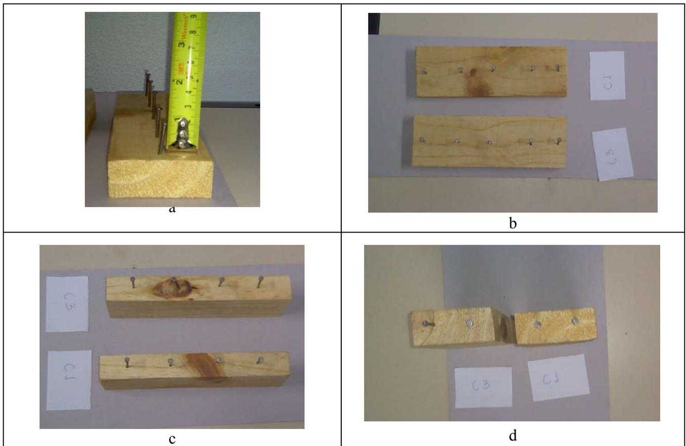
Fig. 4. Holes produced on the surfaces (a) Holes on the largest lateral faces, lateral view; (b) Holes on the largest lateral faces, view from above; (c) Holes on the smallest lateral faces, view from above; (d) Holes on the top and bottom, view from above. Author's collection
