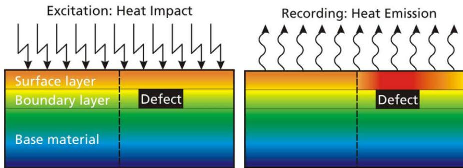
Fig. 1. Principle of infrared thermography, showing the uniformly distributed heat impact on the surface (left), the recorded heat emission (right) and the warmer region (dark) on the surface above the defect, Meinschmidt (2005)
