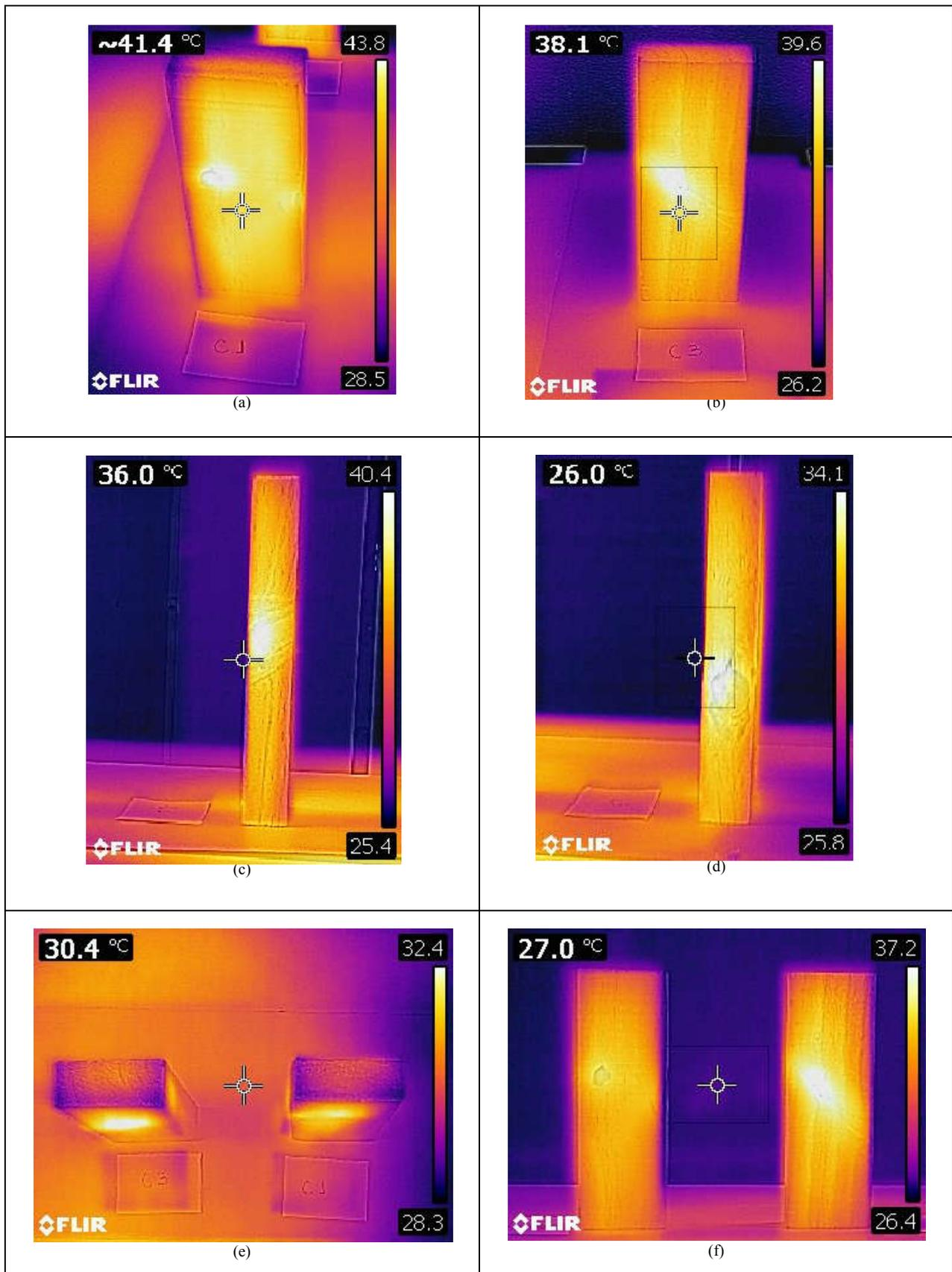
Fig. 6. Cooling process' results, after the 40 minute heating period. Source: Author's collection
